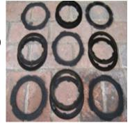
The picture of the smaller multi-spline discs and multi-splined center hub are the 400 turbo. As a matter of explanation, the Watts clutch requires replacing the original large metal discs with fiber discs while the turbo
