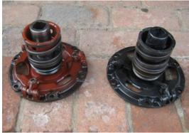
When I removed the old pressure plate and checked the condition of the Watts clutch I discovered the fiber discs were in good condition with the exception of the outer edges where
