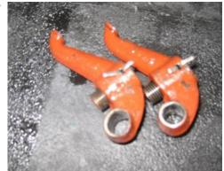
discovered the pressure plate fingers were so badly worn around the pivot holes that I no longer was able to apply even pressure against the discs. You will notice in the picture that the pivot holes were worn thin and the pins were worn as well, which con-
