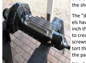
The "dress-up" pieces serve two purposes. One, the aluminum panels have a racy look (for those into that sort of thing) and, two, the ¼ inch thick aluminum is stiffer than the original sheet metal and tends to create a nicer fit. As mentioned in several Ford bulletins, the screws should not be overtightened on the valve cover as it will distort the cover. The aluminum cover poses no such problem nor does the pan inspection cover.
