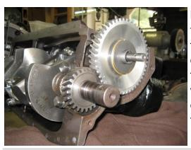
The new cam required a longer front bearing as the front lobe is shorter than the original. I replaced the center bearing as well. Two steel and one bronze thrust washer was added to the front of the camshaft gear, which rests against the inside of the outer cam gear housing and keeps the cam from sliding forward.
