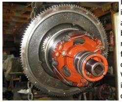
I experienced clutch slippage on the last two tours I participated in. I cranked the set screws down on the pressure plate fingers about as far as I could go and was able to continue on the tours but climbing steep hills became a "religious experience." I was running a Watts clutch and so I thought the problem resided in the
