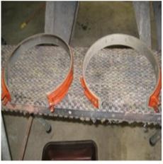
bushings so I think the clutch and transmission problems are now fixed. The Kevlar band lining held up well on the reverse and low gear drums. The brake band on the other hand, not so much. I could have probably removed it and flipped it over but I decided to replace it.
